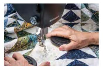
Nina's preferred method of working is to use a BERNINA Gripper Ring. It clearly defines your quilting area. It is weighted and has a gripping surface to manage movement. The quilting area is secured, which prevents the fabric from buckling. Quilt by moving the entire gripper ring.
