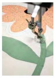
Echo quilting clips are also available. These clips fit onto the ruler foot itself by lowering the foot into the center opening and then pulling it up. This now places the edge of the foot  $\frac{1}{2}$ " from the needle. So, instead of echoing your previous stitching line, you can continue to echo the appliquéd motif. The clips come in three sizes— $\frac{1}{2}$ ",  $\frac{3}{4}$ ", and 1". All three clips have concentric circles, which can be used as further guides.
