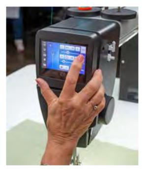
In BSR 2, the needle will rest in an up position versus going continually up and down as it does in BSR 1. Even though the needle is not moving, the machine is still on, as evidenced by the red lights that shine through the quilt sandwich. Take care to avoid placing your fingers in harm's way of the needle when you are ready to resume motion.
