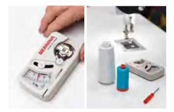
Once a tension of 220 is established, place the bobbin into the bobbin case in the machine's throat plate. Now, the name BERNINA will face out so that you can read it. When you pull on the thread, the bobbin will turn clockwise.
